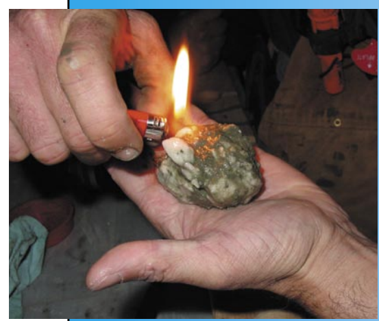
A sample of the sediment that contains methane gas which, when subjected to atmosphere pressure, is liberated and can be used as a source of energy.
